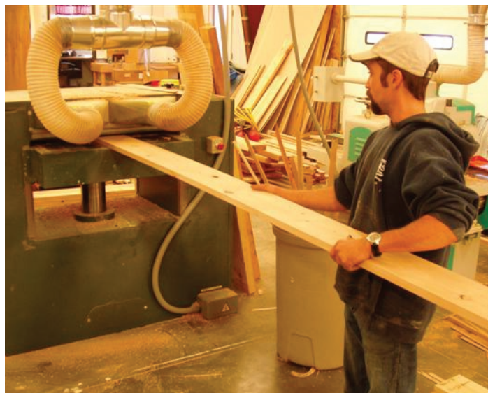
A worker at Intermountain Woodworking feeds materials into the planer to produce a quality board for use in cabinetmaking.
